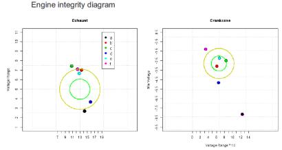
Figure 11: Engine Integrity diagram showing the (dis)similarity of the value of parameters for each cylinder derived from the Signature data.
