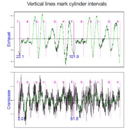
Figure 14: The Polygraph Model of the Pressure vs. vibration in the EP Signature for the subject engine.
